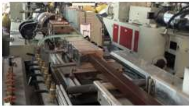
2 Extrusion High-temperature extrusion after compour
