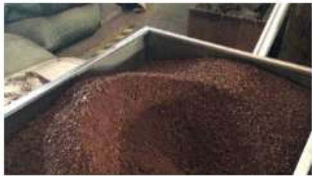
1 Compounding & Pelletizing Recycled HDPE blended with wood fiber.
