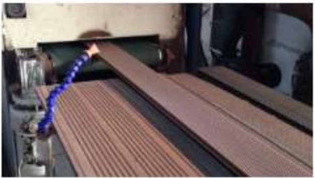
3 Surface Finishing Leveling and texturing the profile surfac
